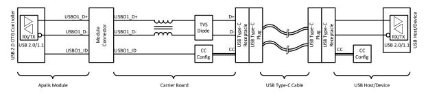
Figure 25: USB-C High-Speed Dual Role (with Type-C connector) block diagram
