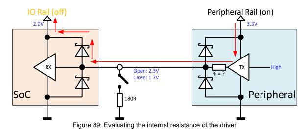
With the help of these formulas, the measured values in Figure 89 would lead to the following internal resistance and backfeeding current:
