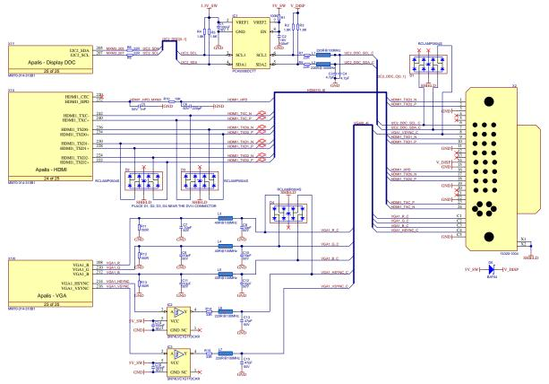
Figure 56: DVI-I reference schematic
