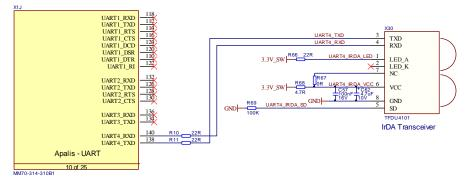
Figure 65: IrDA Reference Schematic
