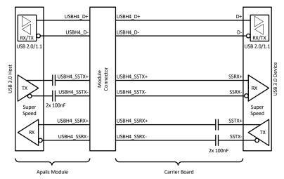
Figure 45: USB 3.x device down block diagram
