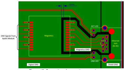
Figure 17: Separation of magnetics ground
