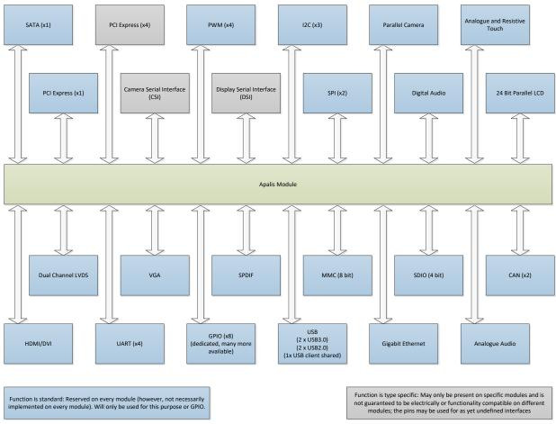
Figure 1: Apalis Module Architecture
