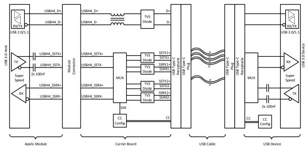
Figure 35: USB-C SuperSpeed DFP-Only (with Type-C connector) block diagram
