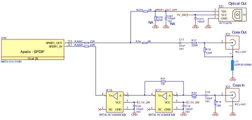
Figure 70: S/PDIF Reference Schematic
