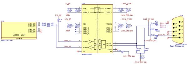
Figure 66: CAN Reference Schematic
