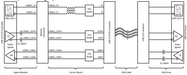
Figure 31: USB 3.x OTG (with Type Micro-AB connector) block diagram
