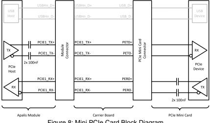
Figure 8: Mini PCIe Card Block Diagram
