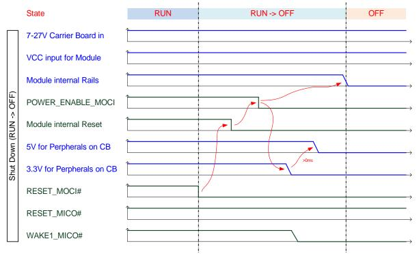
Figure 75: Shut-down sequence
