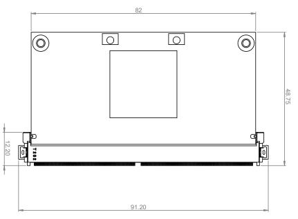
Figure 121: Minimum carrier board space requirement (dimensions in mm)
