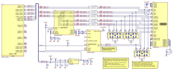
Figure 28: USB-C SuperSpeed Dual Role (with Type-C connector) reference schematic
