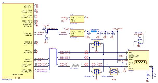
Figure 38: USB 3.x Host-Only (with Type-A connector) reference schematic
