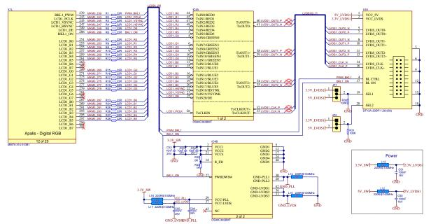
Figure 49: LVDS transmitter reference schematic
