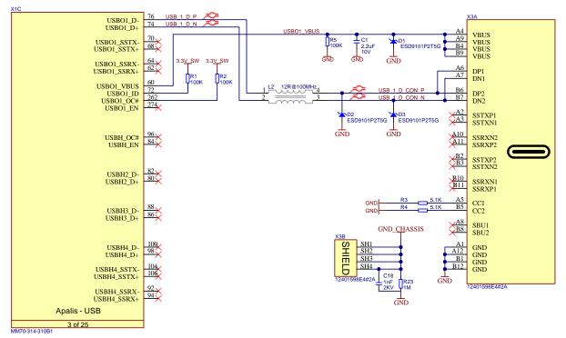
Figure 42: USB-C High-Speed UFP-Only (with Type-C connector) reference schematic
