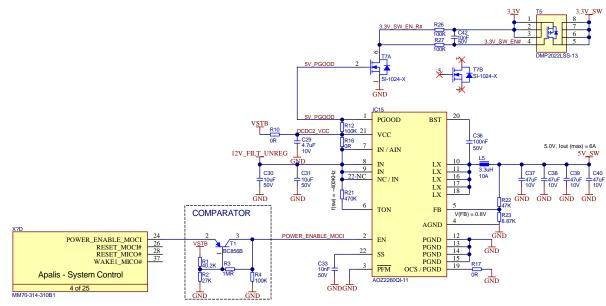
Figure 82: Simple POWER\_ENABLE\_MOCI comparator circuit
