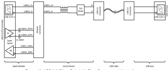
Figure 43: USB 2.0 Client-Only (with Type-B connector) block diagram
