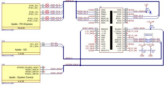
Figure 7: PCIe x1 slot reference schematic
