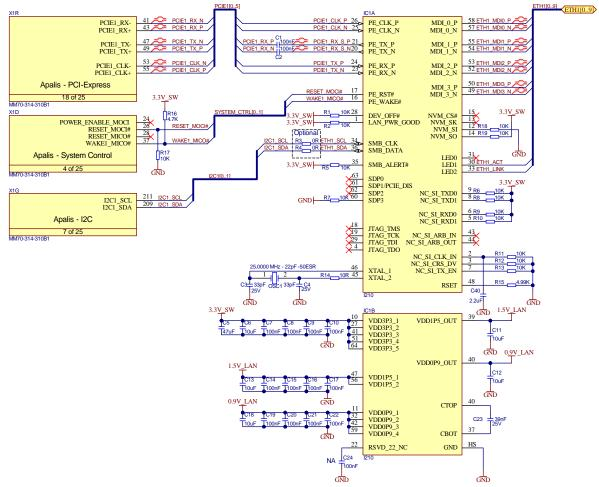
Figure 11: PCIe Device-Down example schematic
