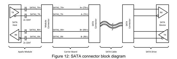
Additionally to the RX and TX pairs, the Apalis module's SATA interface features an LED output signal for signaling activity at the SATA interface (SATA1\_ACT#). The host driver provides this information. The signal type is open drain. Therefore, a pull-up resistor is required on the carrier board. As the signal is used as a signal reference for the SATA1\_TX+ signal in the MXM3 connector, a strapping capacitor of 1nF should be placed from SATA1\_ACT# to GND close to the MXM3 connector.
