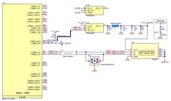
Figure 40: USB 2.0 Host-Only (with Type-A connector) reference schematic
