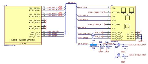
Figure 19: Fast Ethernet with integrated magnetics reference schematic
