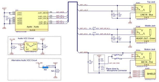
Figure 68: Analogue Audio Reference Schematic
