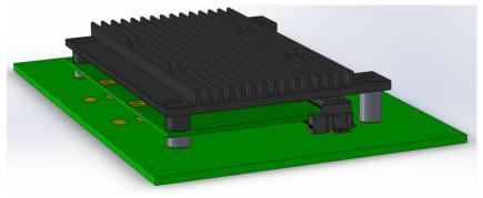
Figure 113: Mounted Heat Sink
