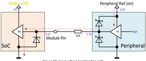
Figure 93: Input without backfeeding path
