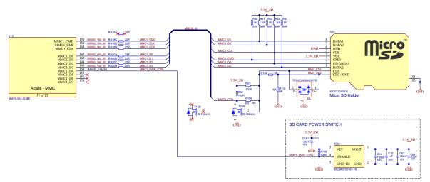
Figure 59: 4bit SD Card Slot Reference Schematic
