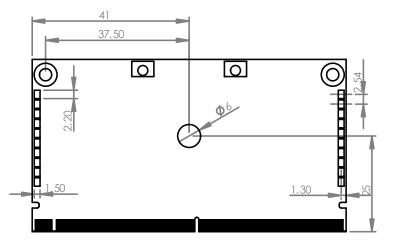
Figure 117: Module dimension bottom side (dimensions in mm)
