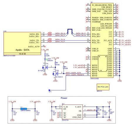
Figure 15: mSATA reference schematic
