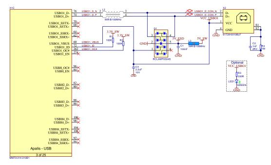
Figure 44: USB 2.0 Client-Only (with Type-B connector) reference schematic
