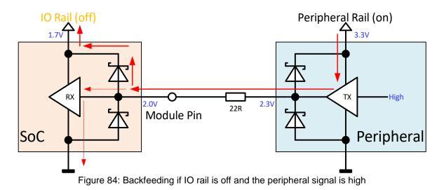
Open drain signals can also cause backfeeding if the pull-up resistor is still powered while the IO rail on the module is off. However, the backfeeding currents are more likely much smaller than with a regular push-pull peripheral output pin. The pull-up resistor value limits the current.
