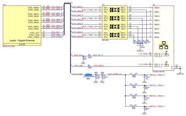
Figure 18: Gigabit Ethernet with discrete magnetics reference schematic
