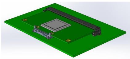
Figure 111: SnapLock fixation
