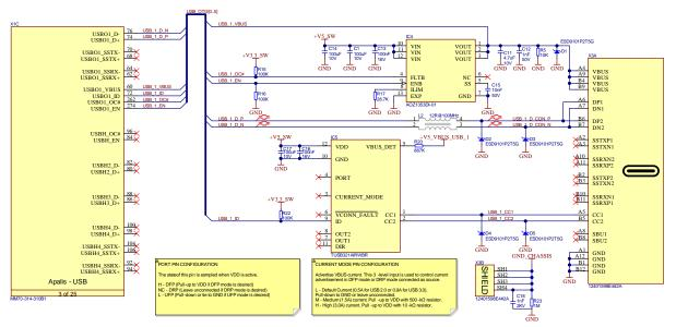
Figure 26: USB-C High-Speed Dual Role (with Type-C connector) reference schematic
