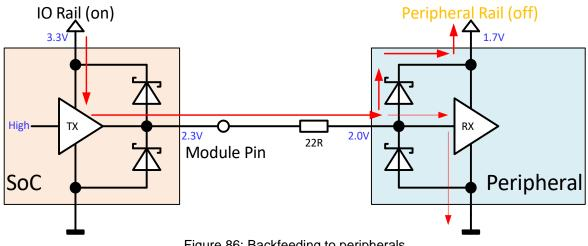
Figure 86: Backfeeding to peripherals
