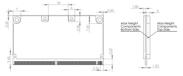
Figure 123: Maximum height of components on module (dimensions in mm)
