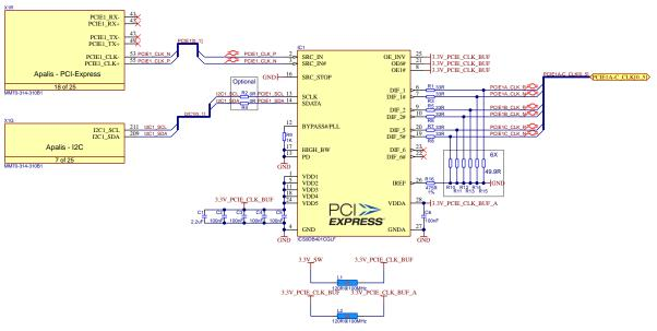
Figure 5: PCIe reference clock buffer example
