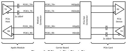
Figure 6: PCIe x1 Slot Block Diagram
