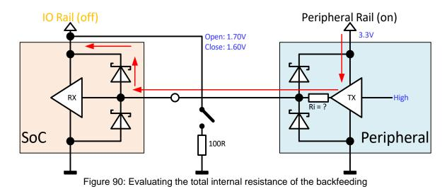
Using the numbers in Figure 90 as an example, we get the following total internal resistance:
