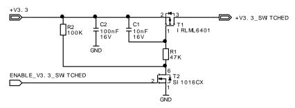
Figure 80: Simple voltage switch circuit
