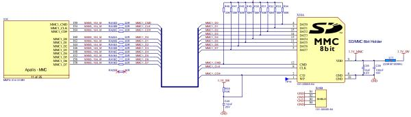
Figure 60: 8-bit MMC/SD Card Slot Reference Schematic
