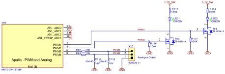
Figure 67: PWM Example Schematic
