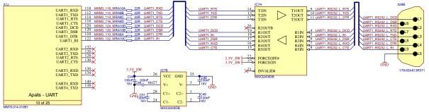
Figure 62: RS232 Reference Schematic
