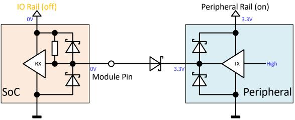
Figure 98: Diode circuit for backfeeding prevention with an on-chip pull-up resistor
