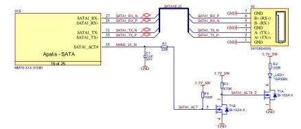
Figure 13: SATA connector reference schematic
