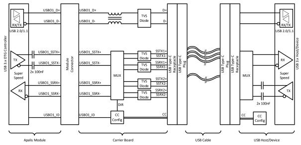
Figure 27: USB-C SuperSpeed Dual Role (with Type-C connector) block diagram
