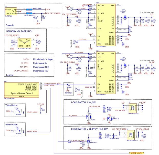
Figure 81: Simple power supply reference schematic
