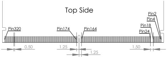
Figure 2: Pin numbering schema on the top side of the module
