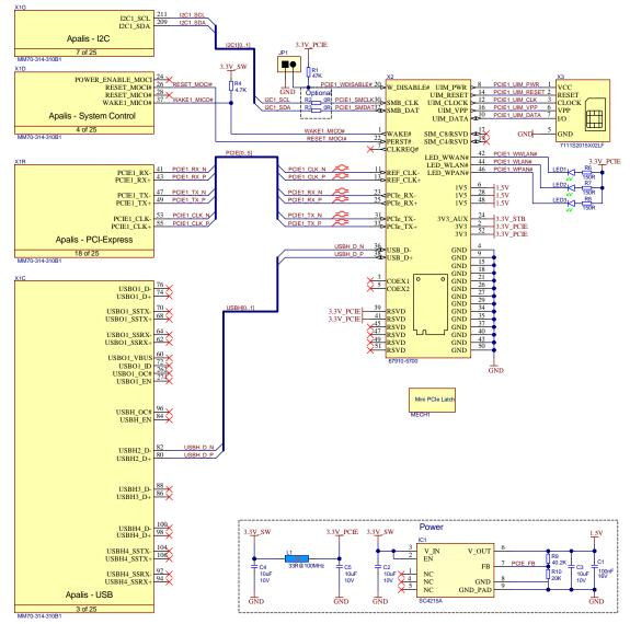
Figure 9: Mini PCIe card reference schematic
