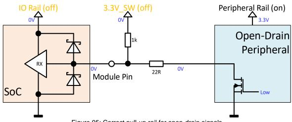
Figure 95: Correct pull-up rail for open-drain signals
