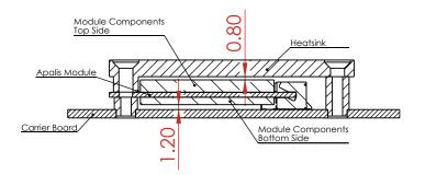
Figure 124: Maximum height of carrier board components under the module
