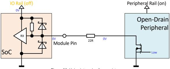
Figure 96: Using internal pull-up resistor
