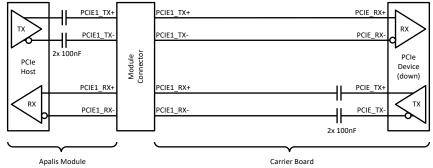
Figure 10: PCIe Device-Down block diagram
