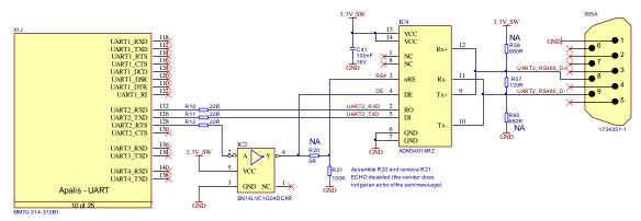
Figure 64: RS485 Reference Schematic
