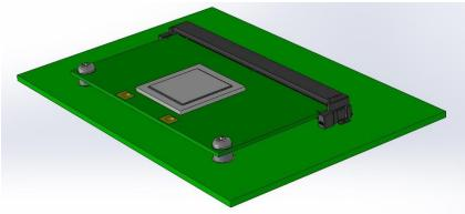
Figure 110: Screw fixation
