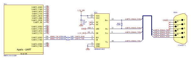
Figure 63: RS422 Reference Schematic
