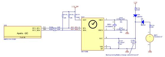
Figure 61: External RTC Reference Schematic
