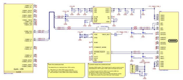
Figure 34: USB-C High-Speed DFP-Only (with Type-C connector) reference schematic
