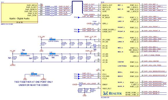
Figure 69: HDA Reference Schematic
