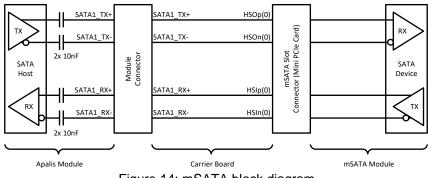
Figure 14: mSATA block diagram
