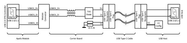
Figure 41: USB-C High-Speed UFP-Only (with Type-C connector) block diagram
