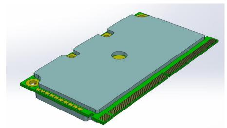
Figure 122: Maximum space requirement of components on module (bottom view)
