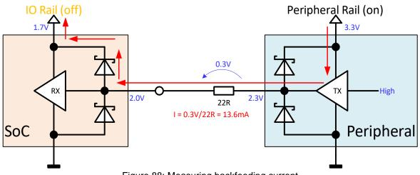
Figure 88: Measuring backfeeding current
